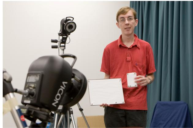
Figure 4b. DisplayObjects configuration, with Vicon cameras and a designer holding the Interaction Palette and a Brick model.
