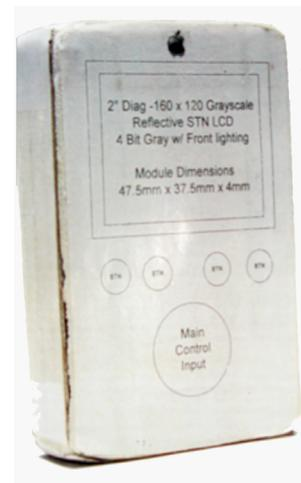
Figure 1. Early Styrofoam mockup of an iPod (courtesy Apple Computers, Inc.)
