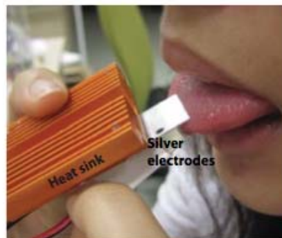
Figure 1. The tongue interface attached to the user's tip of the tongue
