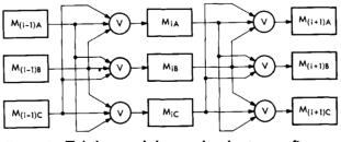
Figure 2 Triple-modular-redundant configuration.
