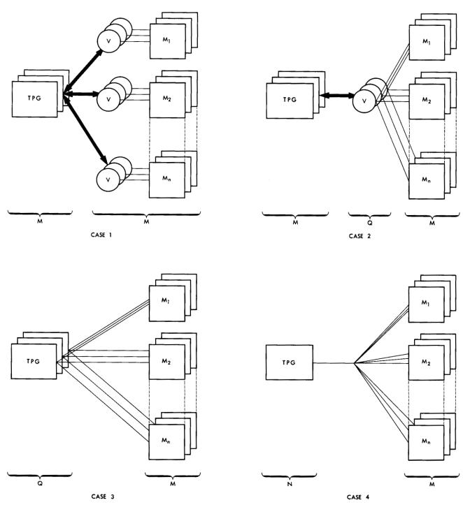
Figure 6 Solutions to problem of unbalance between amount of computer logic and voting logic. + implies that modules are connected to voting circuits as in Fig. 2.
