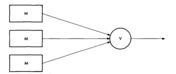
Figure 1 Triple redundancy as originally envisaged by Von Neumann.
