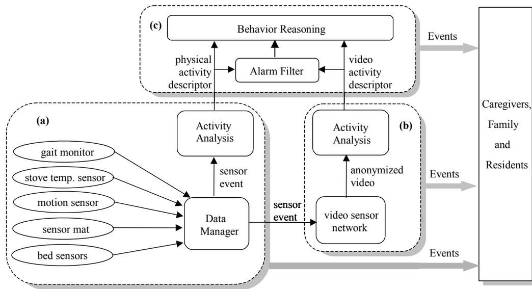
Fig. 1. Components of the integrated monitoring system (a) MARC’s In-home monitoring system (b) Event-driven anonymized video sensor network (c) Recognizing and reasoning about behavioral patterns
