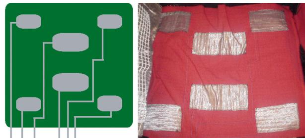
Figure 3. Final seat sensor layout sketch (left), prototype made out of conductive fabric and conductive thread (right)
