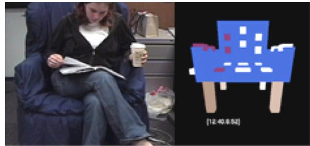
**Figure 4. User in Sense Lounger (left) and visualization of real time sensor data (right). Visualization colors triggered sensors white, and colors the legs according to their pressure.**
