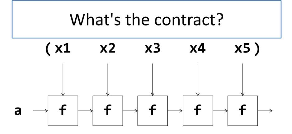
This part is like foldr: We can label all the vertical arrows as X's and all the horizontal arrows as Y's, so the contract becomes (X Y -> Y) Y ListOfX -> Y
